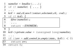
Fig. 8. Extract of parse\_audio\_selector\_unit (From sound/usb/usbmixer.c)
